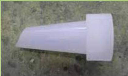
For grouting Vertical Sleeve, cut nozzle on a 45° angle to make a “lip” to insert and rest on the bottom of the inlet tube before raising the pump horizontally and inserting all the way in (see slide 6)
