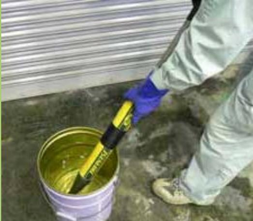
Saturate Pump with clean water to lubricate and help seals.
