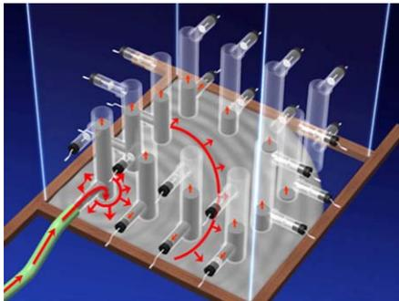
After specially sealing the perimeter of the horizontal joint, the non-metallic SS Mortar® is pumped through a Self Seal Valve in one of the Splice-Sleeve's "Inlet Ports", down into the horizontal joint gap, filling the joint, and then traveling up into all sleeves in one continuous operation. The
